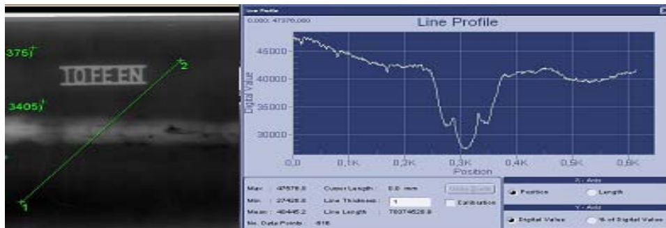
Figure 8. Digital radiography of welded plate with line profile that gives grey counts for part of welding
