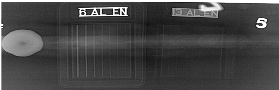
Figure 9. Welded tube Al with diameter 296mm
