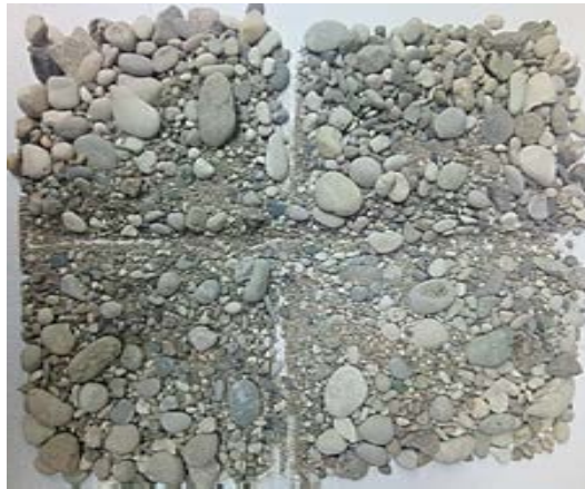
Figure 2.4: Gravel and sand sample for constant head test taken from shallow Holocene Zagreb aquifer
