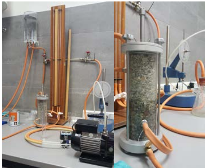
Figure 2.3: Example of the constant head permeameter apparatus (manufacturer: ELE, United Kingdom; Laboratory of the Faculty of Mining, Geology and Petroleum Engineering, University of Zagreb, Croatia)
