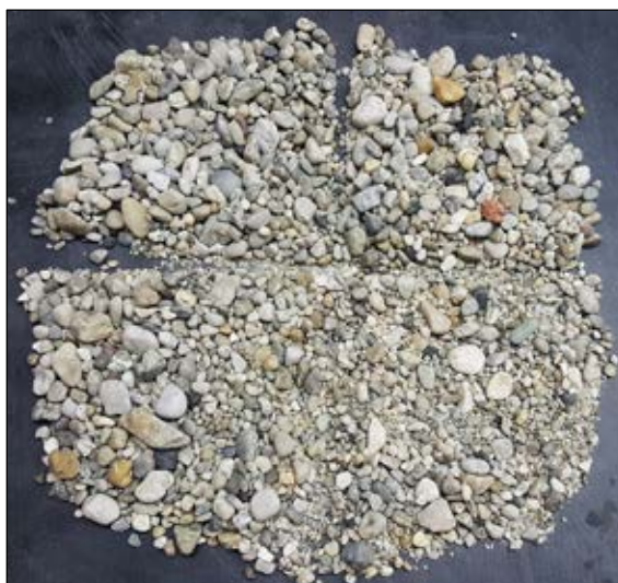
Figure 2.6: Gravel and sand sample for constant head test taken from shallow part of Virovitica aquifer
