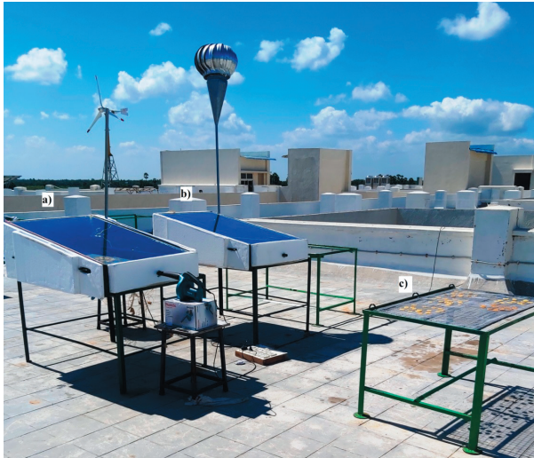
Fig. S1. Photograph of the experimental set-up for banana drying: a) forced convection, b) natural convection single slope solar dryer and c) open sun drying
