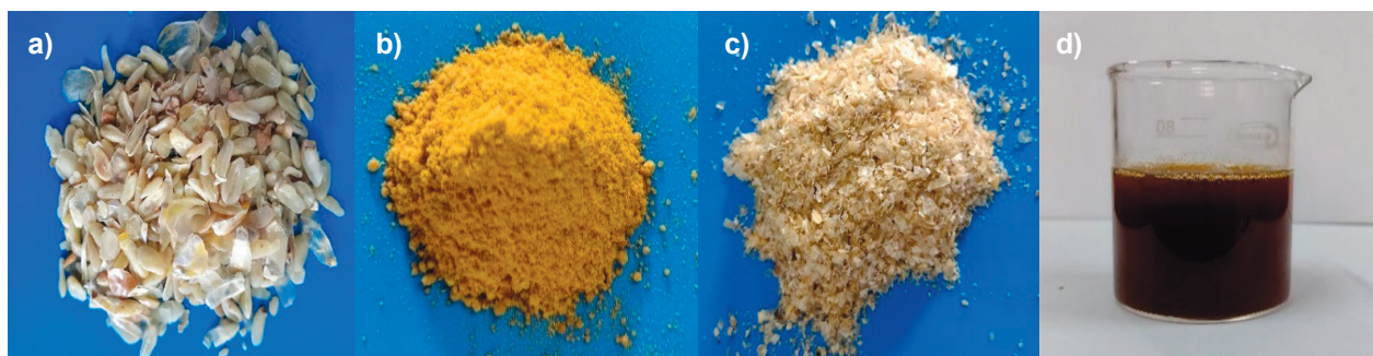
Fig. S1. Industrial maize wet milling by-products: a) maize germ, b) maize gluten, c) maize fibre, and d) corn steep liquor
