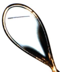
Figure S4. Crystal of \text{Ca}(\text{sac})_2 \cdot 7\text{H}_2\text{O} in the loop used for data collection. Dimensions of the crystal are 0.189 \text{ mm} \times 0.004 \text{ mm} \times 0.004 \text{ mm} . It is elongated along [100] .
