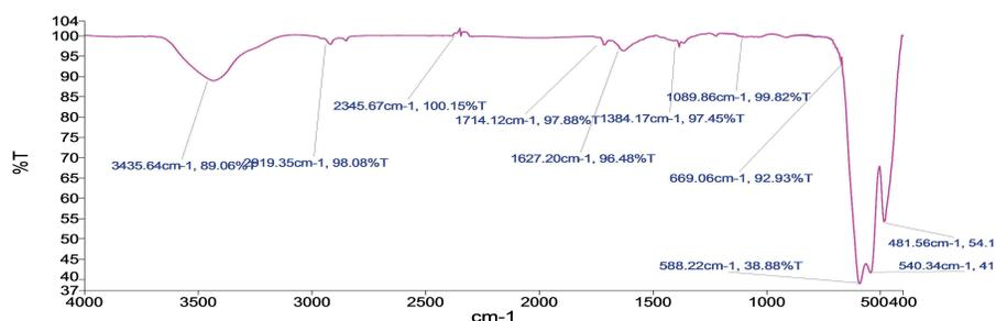
**Figure 1.** FT-IR spectrum of copper ferrite nanoparticles
