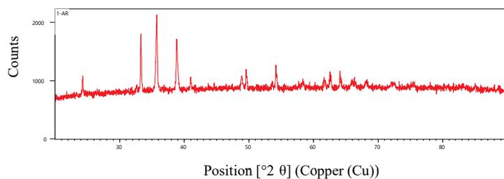
**Figure 2.** X-ray diffraction pattern of  $\text{CuFe}_2\text{O}_4$  nanoparticles
