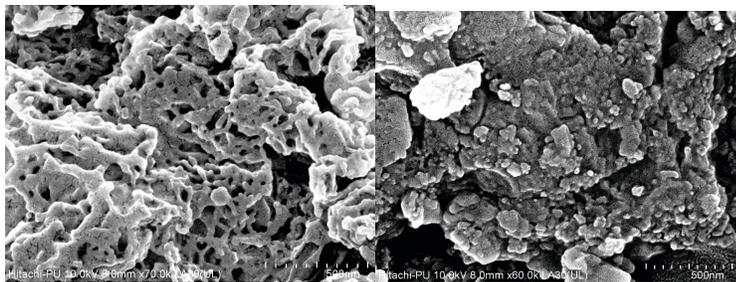
**Figure 3.** SEM images of  $\text{CuFe}_2\text{O}_4$  nanoparticles
