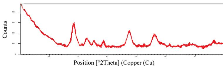
**Figure 4.** X-Ray diffraction pattern of  $\text{CuO-CeO}_2$  nanocomposite
