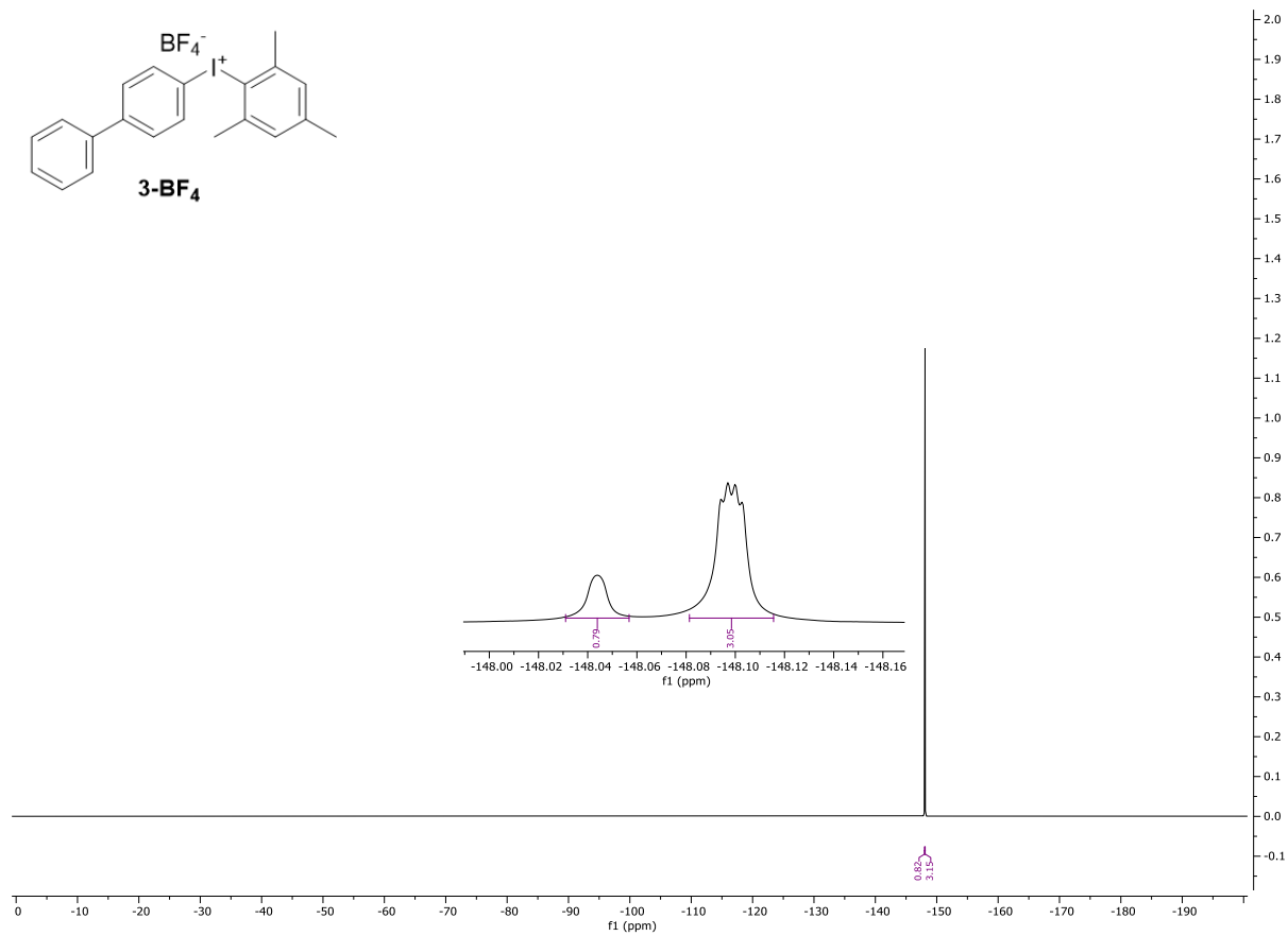
Figure S18. 19 F NMR spectrum (DMSO-d 6 , 376 MHz) of compound 3-BF 4 . The observed splitting in 19 F NMR is due to the 11 B/ 10 B isotope effects.
