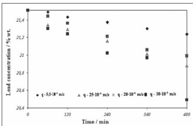
Figure 3 Variation of lead concentration in Cu-Pb-Fe industrial alloy depending on process time
