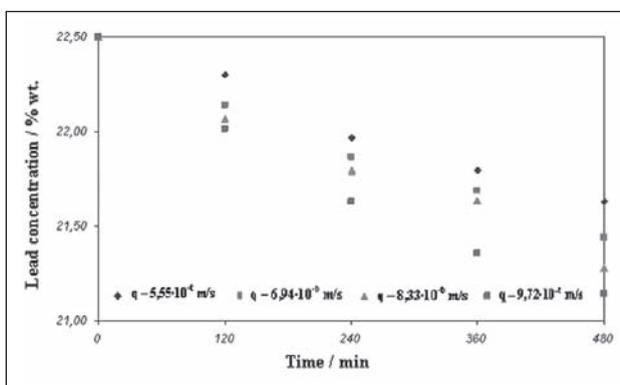
Figure 2 Variation of lead concentration in Cu-Pb-Fe synthetic alloy depending on process time
